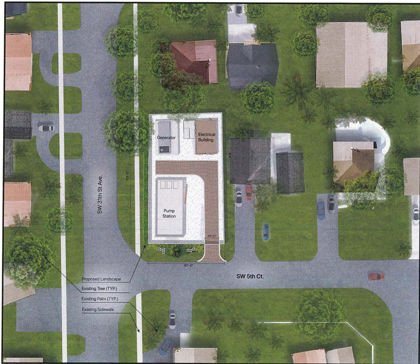
Figure 10: : Proposed Stormwater Pump Station – Option 3 (City Property)
