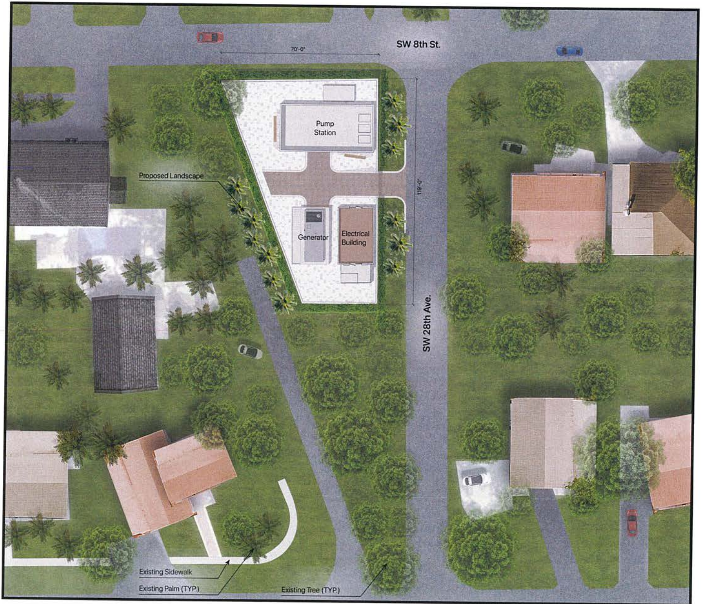
Figure 8: : Proposed Stormwater Pump Station – Option 1
