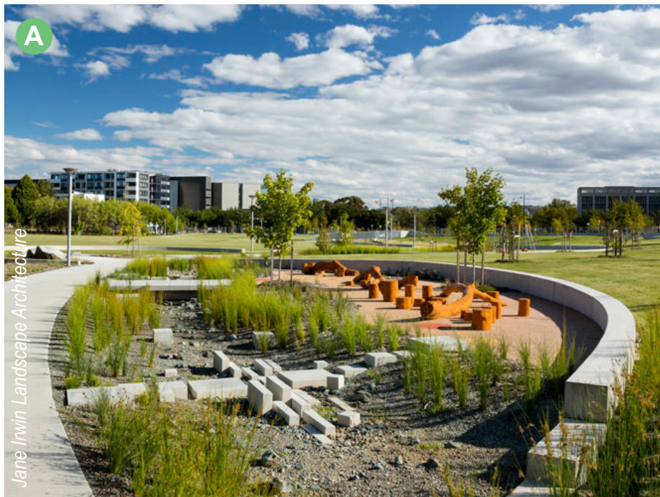
Example of Treatment and Ponding Area Integrated into Park at Hassett Park in Campbell, Australia
